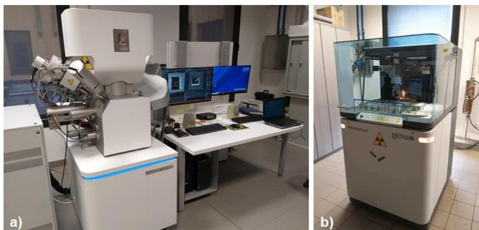
**Figure 6: (a) Dual beam FIB-SEM and (b) XRF spectrometry laboratory for 2D and 3D characterization of geological samples and solid materials at the University of Padova.**
